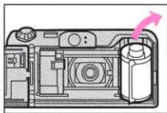
**8. When the film has finished and rewound, remove the film. (→ 23)**
