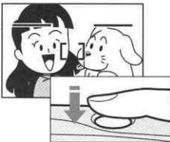
2. Position the AF frame over the subject and hold the shutter button down halfway.
