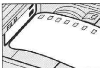
3. Pull the film tip across until it reaches the film tip position mark. Then close the back cover.
