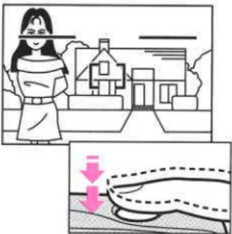
**2. With the shutter button halfway pressed, frame your picture as desired. Then press the shutter button fully.**
