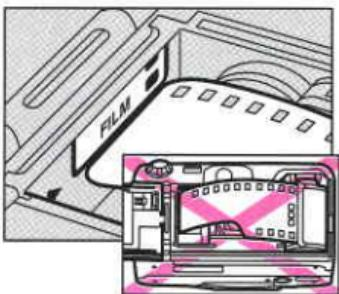
3. Pull the film tip across until it reaches the film tip position mark.
