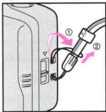
**Pass the strap through the strap holder on the left side of the camera.**
